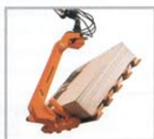
Load sheets vertically and clamp.
